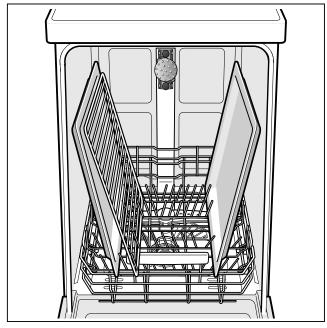
Large sheets or grilles and plates which have a diameter greater than 30 cm (gourmet plates, pasta plates, dinner plates) can be cleaned with the aid of the spray head. To do this, remove the top basket and insert the spray head as illustrated in the diagram.
