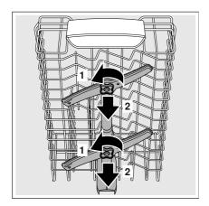
3 Remove the lower spray arm 27 upwards.
